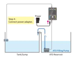
\*The DC pumps can be replaced with larger AC pumps with AUTOAQUA Smart AC Switch
