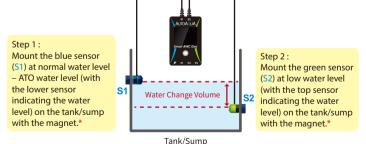
\*Please avoid setting up the sensor in an area with micro bubbles or direct light.
